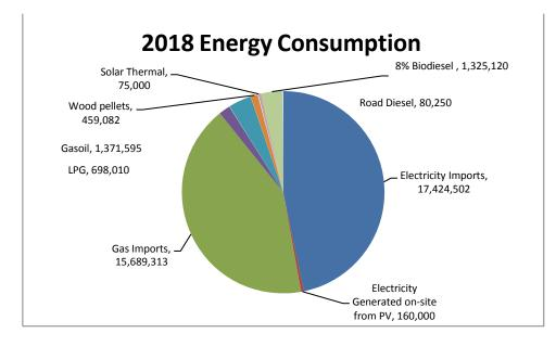
Figure 1: 2018 Breakdown of Energy Consumption (kWh)
